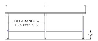
All units ship unassembled for reduced shipping cost. Units 7 ft. and larger are furnished with six legs. All dimensions are typical. Tolerance +/- .500".
