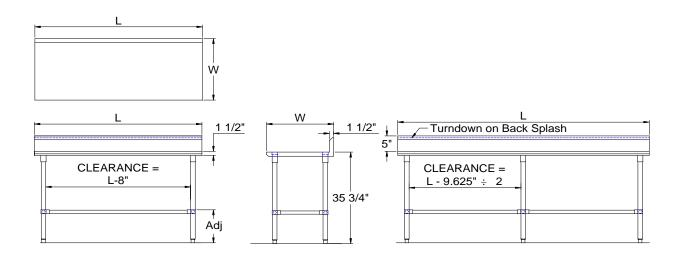
All units ship unassembled for reduced shipping cost. Units 7 ft. and larger are furnished with six legs. All dimensions are typical. Tolerance +/- .500".
