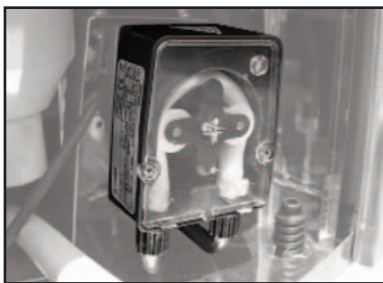
Built-in detergent and rinse chemical pumps.
