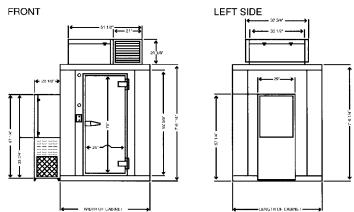
Note: Self-contained units require air circulation around refrigeration system.
