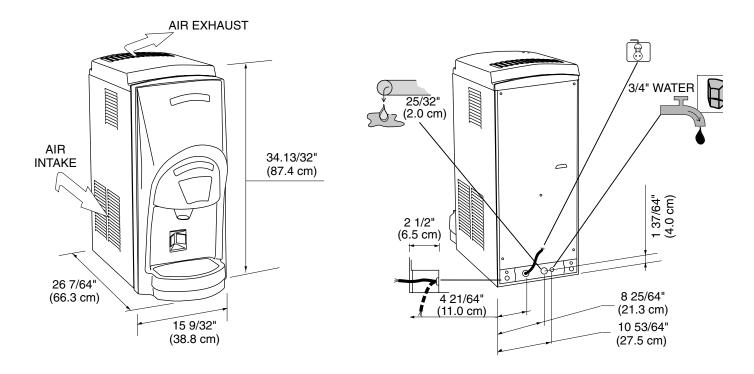
INSTALLATION NOTE: Allow 6" minimum space at left side, top and back for ventilation and utility connections.
