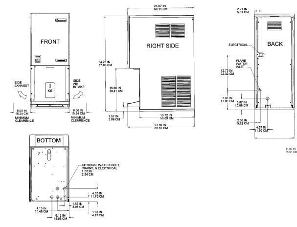
INSTALLATION NOTE: Allow 6" minimum space at sides and back for ventilation and utility connections.
