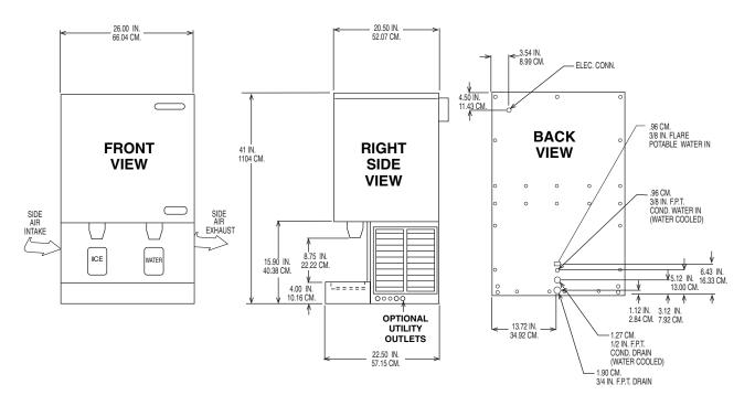
INSTALLATION NOTE: Allow 6" minimum space at sides and back for ventilation and utility connections.
