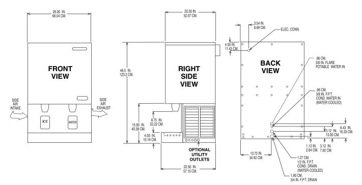
INSTALLATION NOTE: Allow 6" minimum space at sides and back for ventilation and utility connections.
