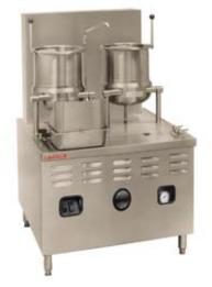
Boiler will be automatically filled with hot water and brought to 15 PSI (*1kg/cm*<sup>2</sup>) pressure when heat and water switches are turned on and automatically drained under pressure when switches are turned off. Automatic cold water condenser will condense exhausted steam into water before releasing it to drain. Unit also includes safety valve, low water cut-off, water strainer, and descaler.
