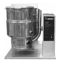
Unit shall be thermostatically controlled to automatically shut off when desired temperature is reached and turn on when product temperature drops below desired setting. Design shall make it possible for one person to easily tilt kettle, even when kettle is filled to capacity. Pouring height allows filling of 4" high pans on the table top. Tilt handle is field reversible for right or left hand tilt.
