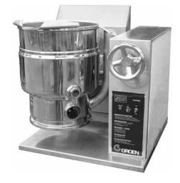
Unit shall be thermostatically controlled to automatically shut off when desired temperature is reached and turn on when product temperature drops below desired setting. Crank tilt design shall make it possible for one person to easily tilt kettle, even when kettle is filled to capacity. Pouring height allows filling of 4" high pans on the table top.
